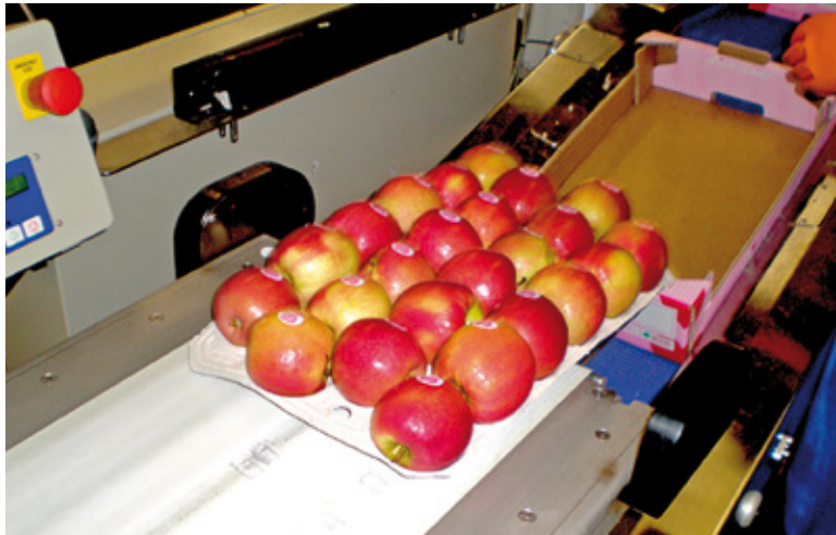
Soft infeed of trays in carton boxes or plastic crates by telescopic system
